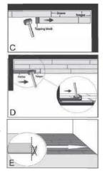
3) Irregular wall along the first row of planks - scribe the planks to fit the wall and cut.
