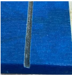
First - Backside cut ½ depth
