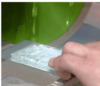
Wet Saw cutting full depth through face
